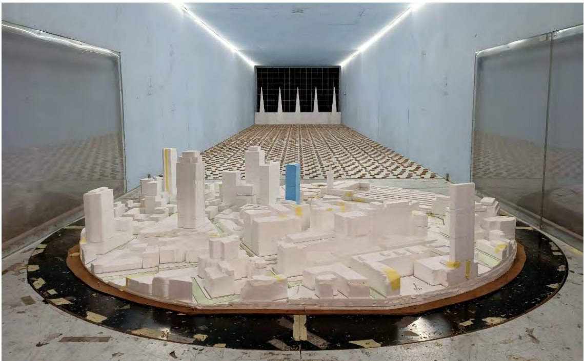
Figure 1f: Photograph of the Wind Tunnel Model (Proposed Case, view from the west)
