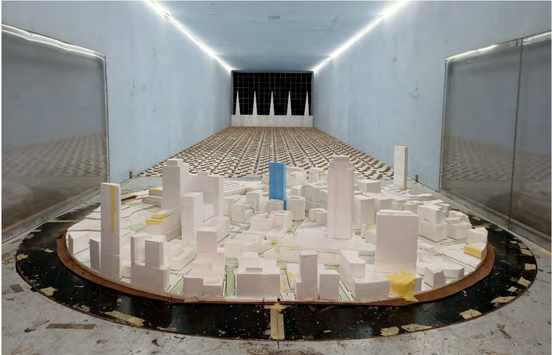
Figure 1g: Photograph of the Wind Tunnel Model (Proposed Case view from the north)
