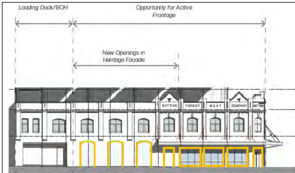
Figure 25 Vehicular Entrance off Valentine Street and Continuous Active Frontage Source: Grimshaw
